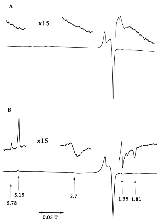
FIGURE 2: Electron flux dependency of the EPR spectrum of hi-CO. Experimental conditions: (A) [Av2]/[Av1] = [8 \mu M]/[40 \mu M] = 1:5; [CO] = 1 atm; [ATP] = 12.5 mM (5 \times normal concentration); [MgCl 2 ] = 25 mM; [Na 2 S 2 O 4 ] = 20 mM; 50 mM TES-KOH, pH 7.4; following a 10 min incubation at 30 ^{\circ} C, samples were rapidly frozen in liquid N 2 ; (B) conditions identical to those in (A) except that [Av2]/[Av1] = [40 \mu M]/[40 \mu M] = 1:1. Spectrometer parameters: microwave frequency = 9.44 GHz; microwave power = 15 mW; center field = 0.26T; field sweep = 0.32 T; modulation amplitude = 0.5 mT; Temperature = 8 K; inserts in (A) and (B) at gain 15 \times that used for full spectra.
